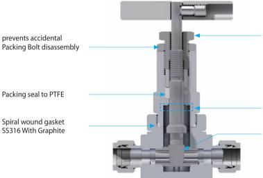
Packing bolt design permits packing adjustments in the open position
